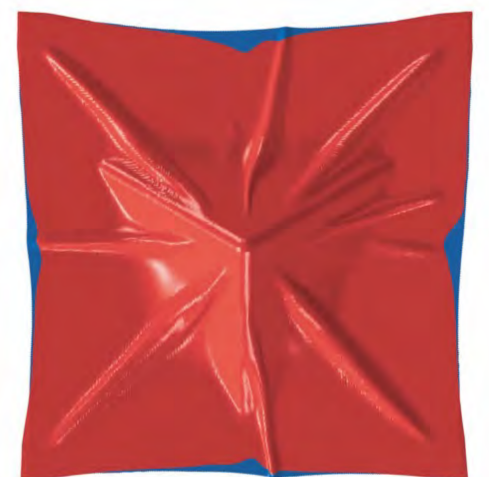
Comparison of multi-layer forming experiments with simulation for Double Diaphragm forming processes
