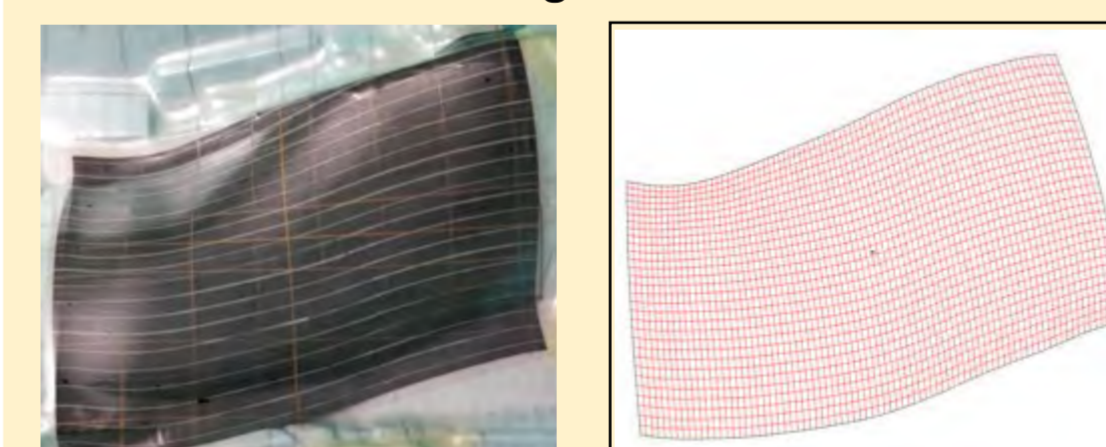
Figure 7. Comparison between Formed tailored CTS prepreg and Reformed preform with tailored fibre path
