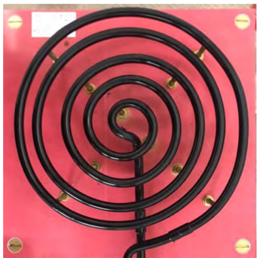
Above: (Left) Photograph showing standard pancake coil design used for metallic processing. (Right) Thermal image showing the ring shaped heating pattern produced using the pancake coil.
