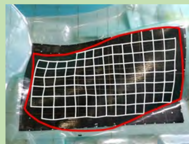
Figure 2. experimental results (left) of forming using UD prepreg with marked grids and model prediction (right) for the re-forming of prepreg tailored fibre path
