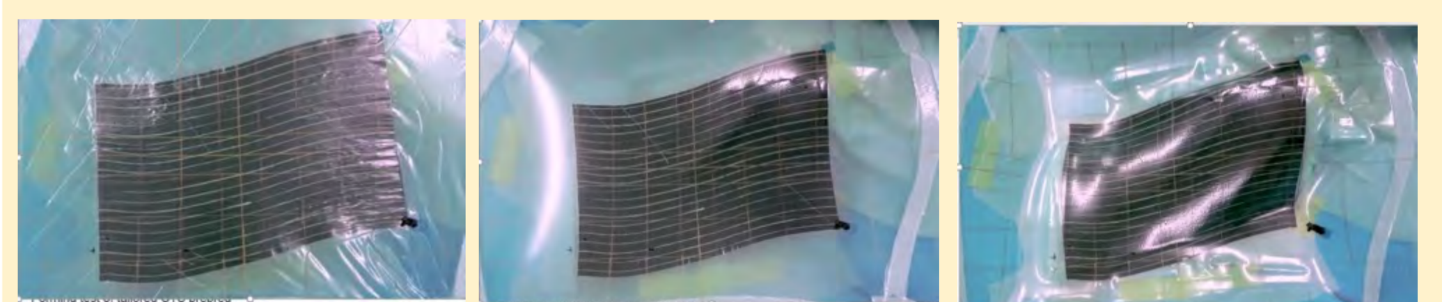
Figure 6. Double diaphragm forming test on tailored CTS prepreg where fibre path was derived from un-forming simulation
